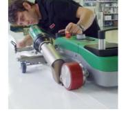
Very easy hem and piping welds with the hem/piping welding kit
