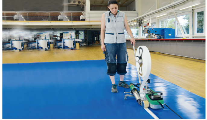
An economical, ergonomic tool for welding reinforcement tapes.
